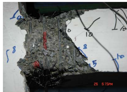
Fig. 5: Test Specimens; C2 at failure
